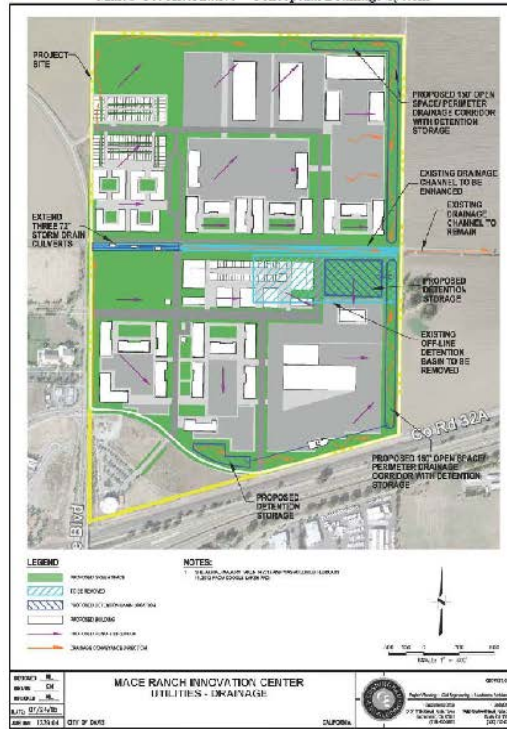
Figure 8-9 Mixed Use Alternative - Conceptual Drainage System
